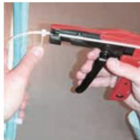
Grip the cable tie with the tool.
