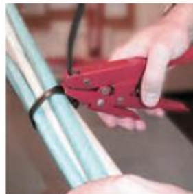
Tighten the tie till the complete fixing.
