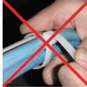
Avoid sharp bending of the tie: it will not improve the fixing strength.
