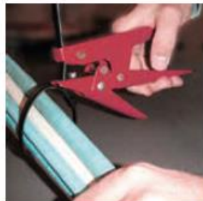
Use the tool for tightening the tie around the cables.
