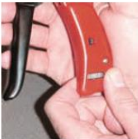
Set the max tension of the tool depending on the size of the tie.
