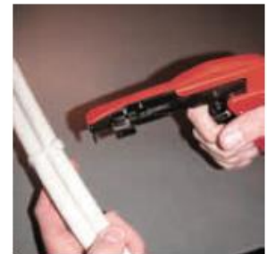
Cut the exceeding part of the cable tie, properly adjusting the setting of the tool.
